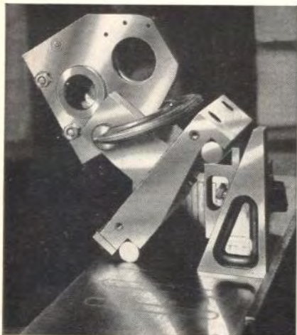
Used in Conjunction with Sine Bar in Grinding Angles
